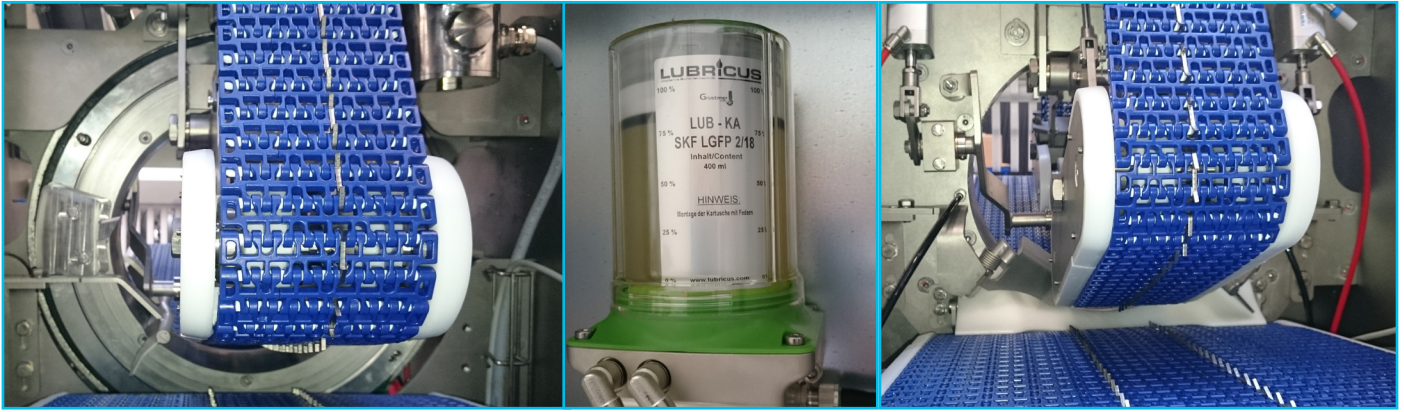
New design on pressure wheel as well as indication by empty lubrication container
